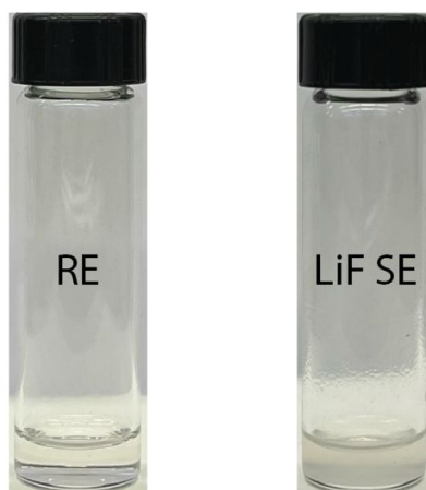
Figure S1. Photographs of RE and LiF SE taken after resting the electrolytes for a day. LiF SE exhibits an opaque solution.
